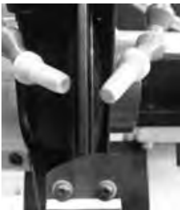
Knife rest and grinding wheel for sharpening blade in a Helicarb cutter on a Weing Rondamat Grinder or equivalent.
